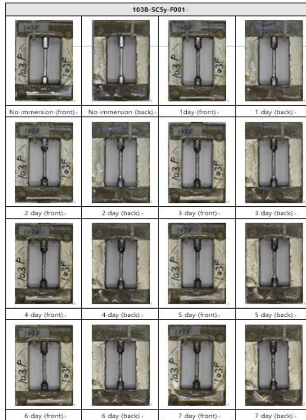
• ASTM G47, 7075 stress corrosion cracking
